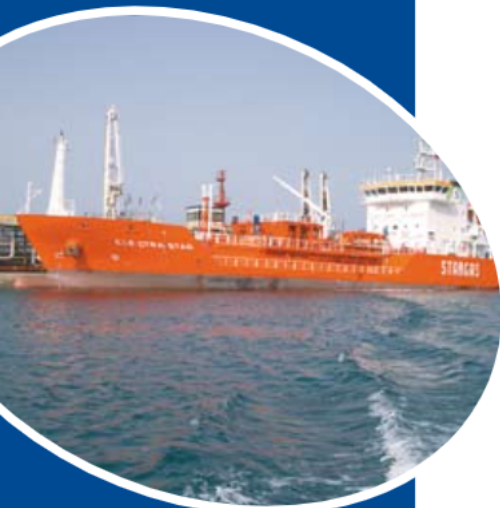
1290 kW LPG Cargo Condenser on LPG Vessel, PSHE 9LL-222/1/1 (titanium plates)
